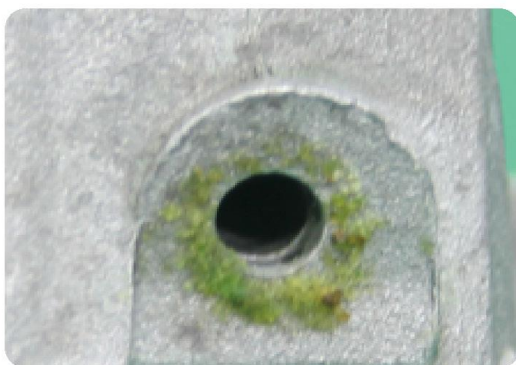
Traces of dried coolant are normal.
